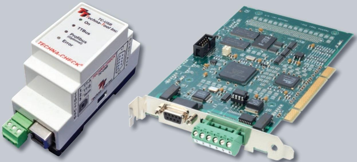
These systems use USB or PCI to interface with a Windows based CNC control or into a stand-alone computer. They are capable of monitoring up to 128 different cutting processes per sensor and can network up to 20 sensors/channels back to a single unit.
